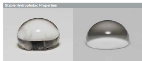
Water droplet on a dirty silicone coating.
