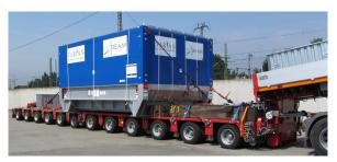
The heavy cargo logistic provider Arnold Schwerlast GmbH & Co. KG was in charge of the transport of the 100 ton heavy Cyclotron from Cologne/Germany to San Diego/USA.
