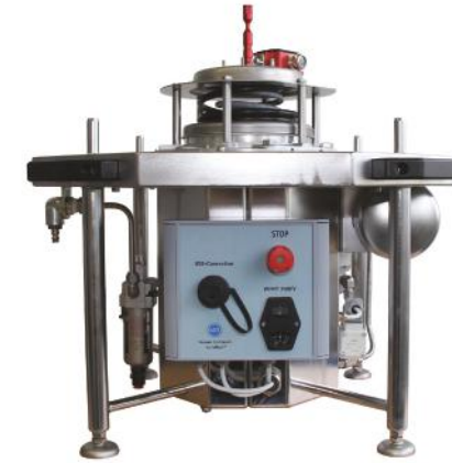
MPreC® test bench with installed pressure relief device
